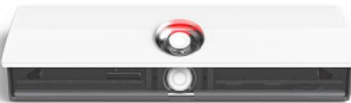
Hob Guard works by means of four sensors which monitor's the hob constantly, raising a pre warning 15 second alarm when conditions approach an unacceptable level. Where no action is taken or conditions become critical, the Hob Guard is activated in fire mode to prevent the fire occurring.
